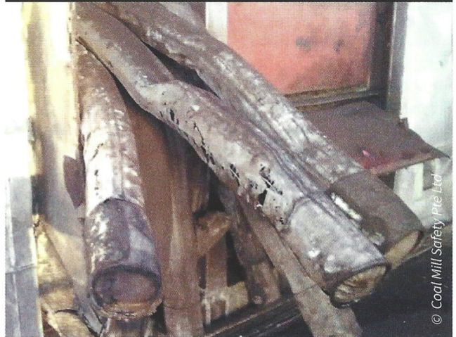
Figure 1: example of incorrect explosion protection design: non-self-reclosing explosion vents, filter cages and bags in the way of venting blasts
